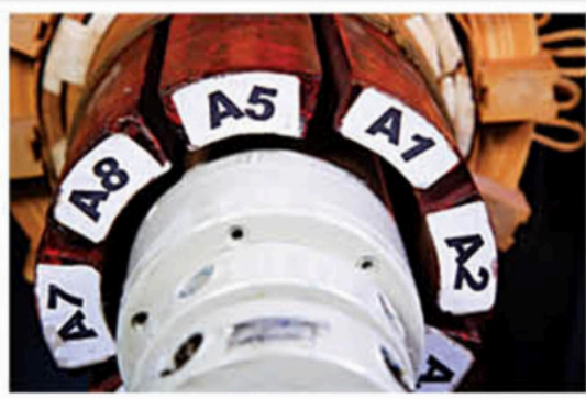
Collapsible Former – Helps in cutting short of winding time.
