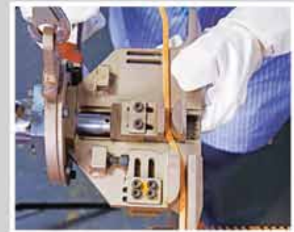
S Bend Tool – Intricate S or Z bends can be achieved easily and smoothly
