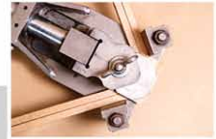
90° Start Bend Tool - Easier bending operation on conductors eliminating cracked surfaces
