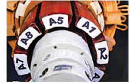
Collapsible Former – Helps to shorten the winding process
