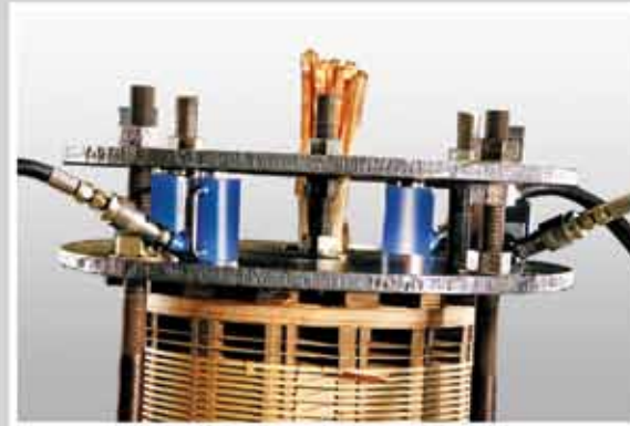
Coil tightening to the designed pressure with a hydraulic system
